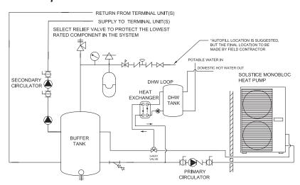
\*Autofill system is suggested but not required by SpacePak. If such installation is desired or required by local code, the Autofill MUST draw from a reservoir of pre-mixed glycol/water solution. Filling directly from a well or municipal water source may introduce contaminants and will dilute the glycol solution in the event of a system leak. This may impact warranty coverage.
